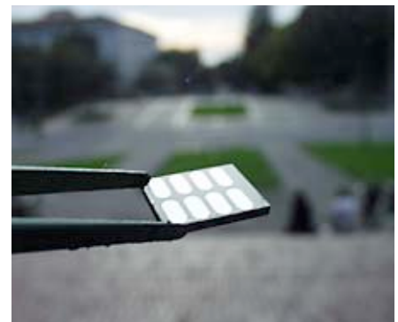
Picture of a solar cell, which utilizes nanorods to convert light into electricity (Ref. 5).
